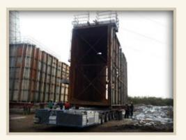
In an effort to become more diversified and enter into newer markets, PSC Crane & Rigging has purchased a Goldhofer PST/SL-E 6-12x08. This Self Propelled Electronic Steer 6 axle module is capable of handling 40 ton per axle. The power-pack is designed to run a total of 46 lines in several configurations. This type of equipment will definitely assist us on large press projects as well as in the energy production industry.
