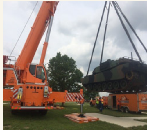
PSC lifting and setting a 117,000 lbs. M1 Abrams Tank
